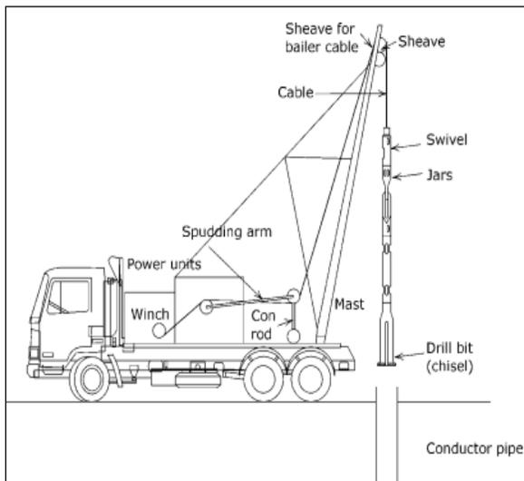
*Figure 3.1a: Percussion drilling rig*
